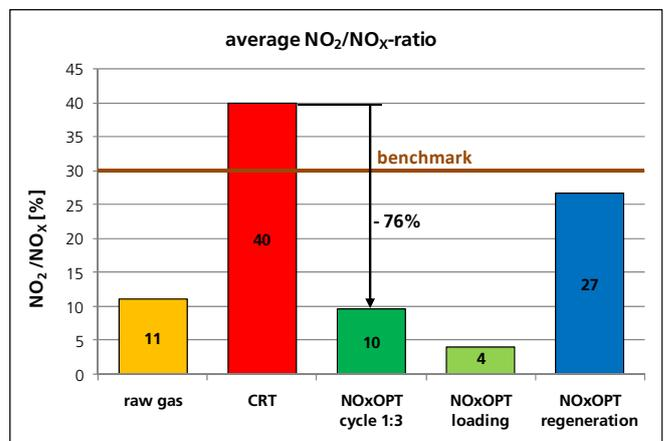
Fig. 5: average NO<sub>2</sub>/NO<sub>x</sub>-ratio under field conditions
