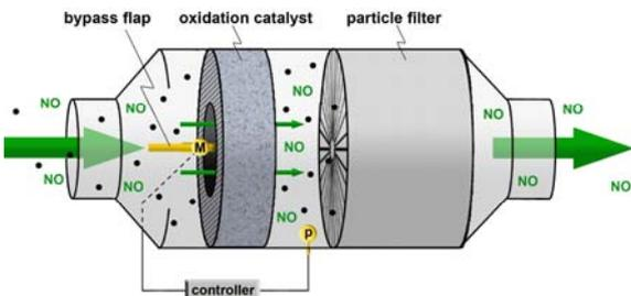
Fig. 2: load operations (flap opened)
