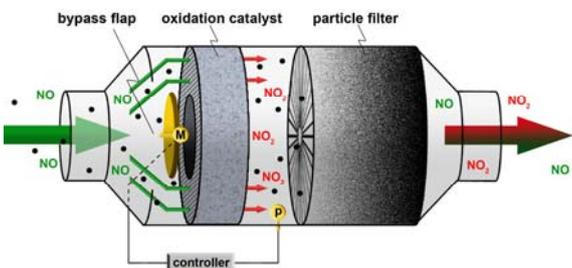
Fig. 3: regeneration operations (flap closed)
