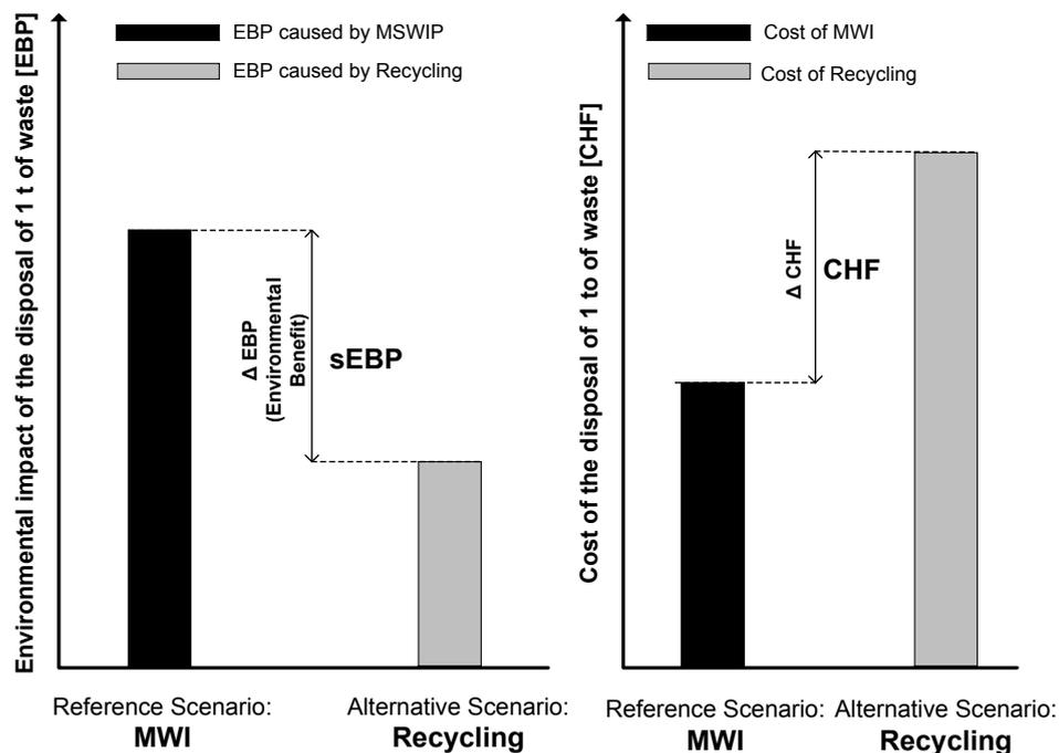
**Fig. 3:** "Reference Scenario" municipal solid waste incineration MSWI vs. "Alternative Scenario" recycling. Left: Quantification of environmental burden by environmental burden points leads to  $\Delta EBP$ . Right: In the same way, the costs ( $\Delta CHF$ ) which are additionally incurred against a reference scenario are determined. These two differences ( $\Delta EBP$  and  $\Delta CHF$ ) are divided to determine the SEBI:  $SEBI = \Delta EBP / \Delta CHF = sEBP / CHF$ .
