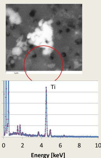
Figure 6: top: Backscattered electron (BSE) image of a TiO<sub>2</sub> particle recorded at higher magnification. Bottom: Respective EDX spectrum.
