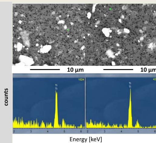
Figure 5: top: Backscattered electron (BSE) image resulting from CC-SEM. Bottom: EDX spectra of TiO<sub>2</sub> particles detected by CC-SEM.
