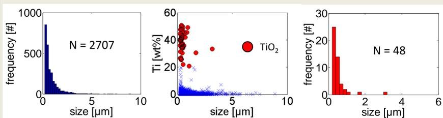
Figure 4: A: Particle size distribution of all particles detected using computer controlled scanning electron microscopy. Larger particles were removed previously by sedimentation. B: Size vs. Ti content of all particles. The TiO<sub>2</sub> particles are marked in red. C: Size distribution of TiO<sub>2</sub> particles.
