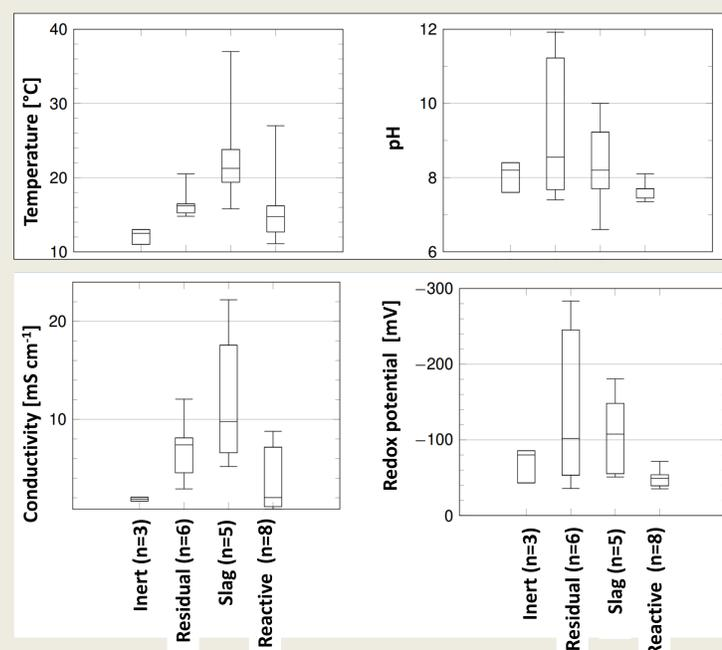
Figure 3: Temperature, pH, conductivity and redox potential measured in the leachates of the selected landfills
