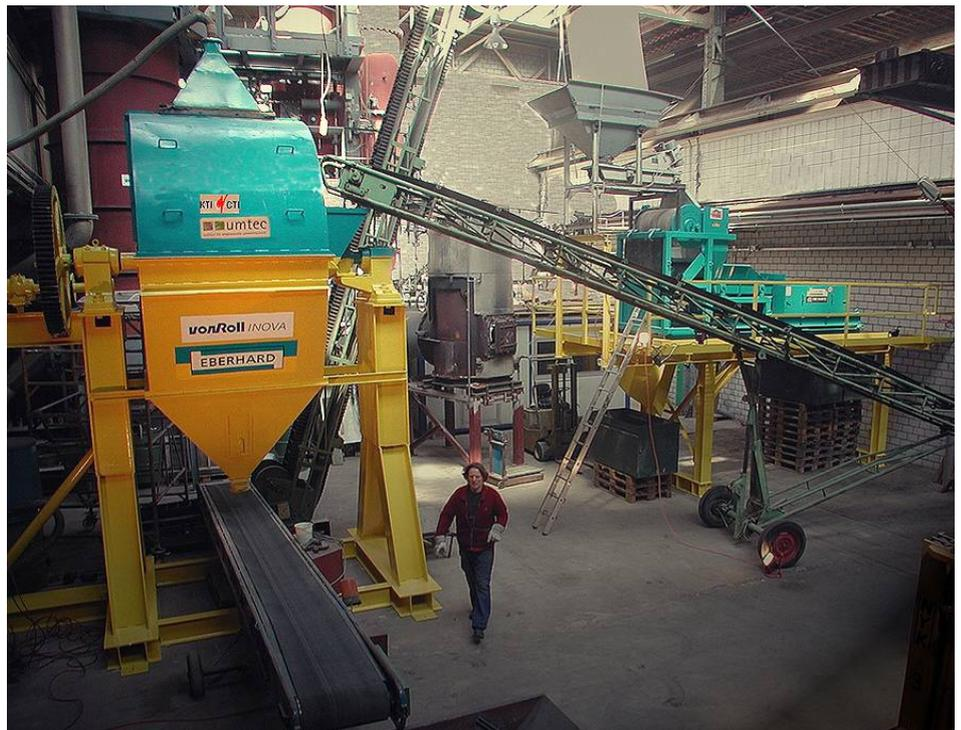
Fig. 1: pilot installation for bottom-ash processing; operator UMTEC / von Roll Inova / ERAG
