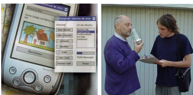
Fig. 4: pda micro-computer with software for odour monitoring
