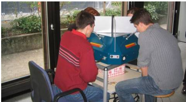
Fig. 1: four test persons deployed at an olfactometer of UMTEC
