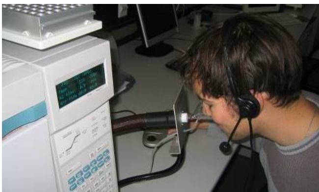
Fig. 2: sniffing the odour-active components of a gas mixture at the "sniffing port" of our gas chromatograph
